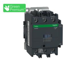
contactor, TeSys Deca, 3P(3NO), AC-3/AC-3e, <=440V, 80A, 380V AC 50/60Hz coil
