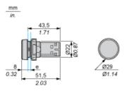
Support panel thickness: 1 to 6 mm/0.4 to 0.24 in. (metal), 2 to 6 mm/0.8 to 0.24 in. (plastic).
