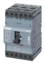
circuit breaker 3VT1 standard breaking capacity Icu=25kA, 415V AC 3-pole, line protection trip unit TM, LI In=16A rated current IR=12.5...16A overload prot. II=160...240A, short-circuit protection without auxiliary release without auxiliary/alarm switch
