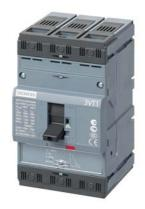
circuit breaker 3VT1 standard breaking capacity Icu=25kA, 415V AC 3-pole, line protection trip unit TM, LI In=20A rated current IR=16...20A overload protection II=200...300A, short-circuit protection without auxiliary release without auxiliary/alarm switch
