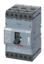
circuit breaker 3VT1 standard breaking capacity Icu=25kA, 415V AC 3-pole, line protection trip unit TM, LI In=25A rated current IR=20...25A overload protection II=250...375A, short-circuit protection without auxiliary release without auxiliary/alarm switch
