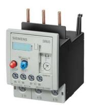
Overload relay 36...45 A For motor protection Size S2, Class 10 Contactor mounting Main circuit: Screw terminal Auxiliary circuit: Screw terminal Manual-Automatic-Reset !!! Phased-out product !!! Successor is SIRIUS 3RU2 Preferred successor type is >>3RU2136-4GB0<<
