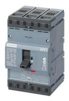
circuit breaker 3VT1 standard breaking capacity Icu=25kA, 415V AC 3-pole, line protection trip unit TM, LI In=40A rated current IR=40A overload protection II=160A, short-circuit prot. without auxiliary release without auxiliary/alarm switch
