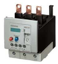
Overload relay 57...75 A For motor protection Size S3, Class 10 Contactor mounting Main circuit: Screw terminal Auxiliary circuit: Screw terminal Manual-Automatic-Reset !!! Phased-out product !!! Successor is SIRIUS 3RU2 Preferred successor type is >>3RU2136-4RB0<<
