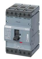
circuit breaker 3VT1 standard breaking capacity Icu=25kA, 415V AC 3pole, line protection trip unit TM, LI In=63A rated current IR=63A overload protection II=252A, short-circuit prot. without auxiliary release without auxiliary/alarm switch
