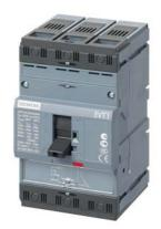
circuit breaker 3VT1 standard breaking capacity Icu=25kA, 415V AC 3-pole, line protection trip unit TM, LI In=80A rated current IR=80A overload protection II=320A, short-circuit prot. without auxiliary release without auxiliary/alarm switch
