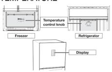
We recommend setting the temperature of the freezer and the refrigerator to **Optimal** to ensure a stable performance of the appliance.
